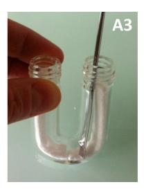
Then, put 1 mL odorous solution on each piece of polypropylene (2 mL in total in the tube). This needs to be done cautiously with a pipette, in such a way that the liquid is deposited only on the polypropylene (not on the tube) and all along it from bottom to top to ensure optimal absorption (see Fig. B1-2).
