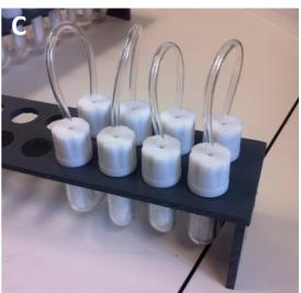
Finally, plug the tubes (insert a seal between the plug and the top of the tube to ensure airtightness) in the tube rack and close them (see Fig C) with a flexible tube.
