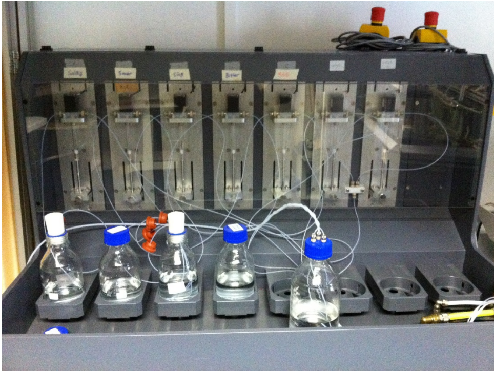
Fig. 1.7: Computer controlled gustometer. The different taste-solutions are filled into separate pipettes. The tastants are delivered to the subject with exact timing and portioning, as determined by the sequence pre-programmed in the computer. Photo: C. Enger (2017).
