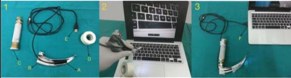
Fig. 1 Device assembled using an USB camera (A), Macintosh laryngoscope blade (B), handle (C), Durapore adhesive tape (D). The camera is interfaced to a personal computer USB port (F) using its connector (E) and visual orientation is checked during assembly
